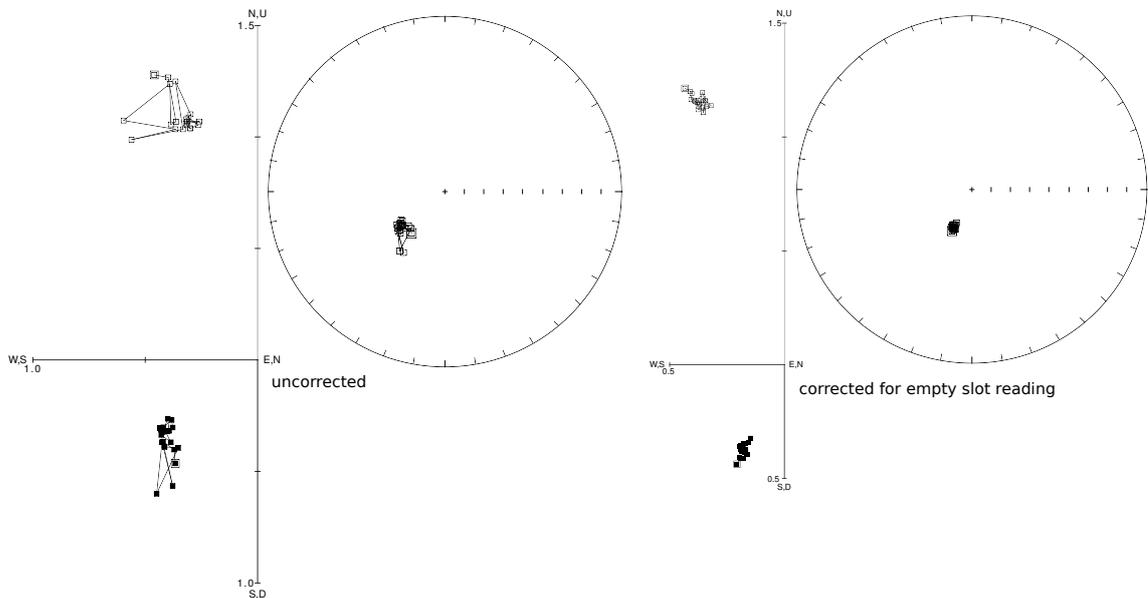
**Figure 9** Effects of subtracting measured magnetization of empty slot (position 7) from that of Sample 4 (position 8).
