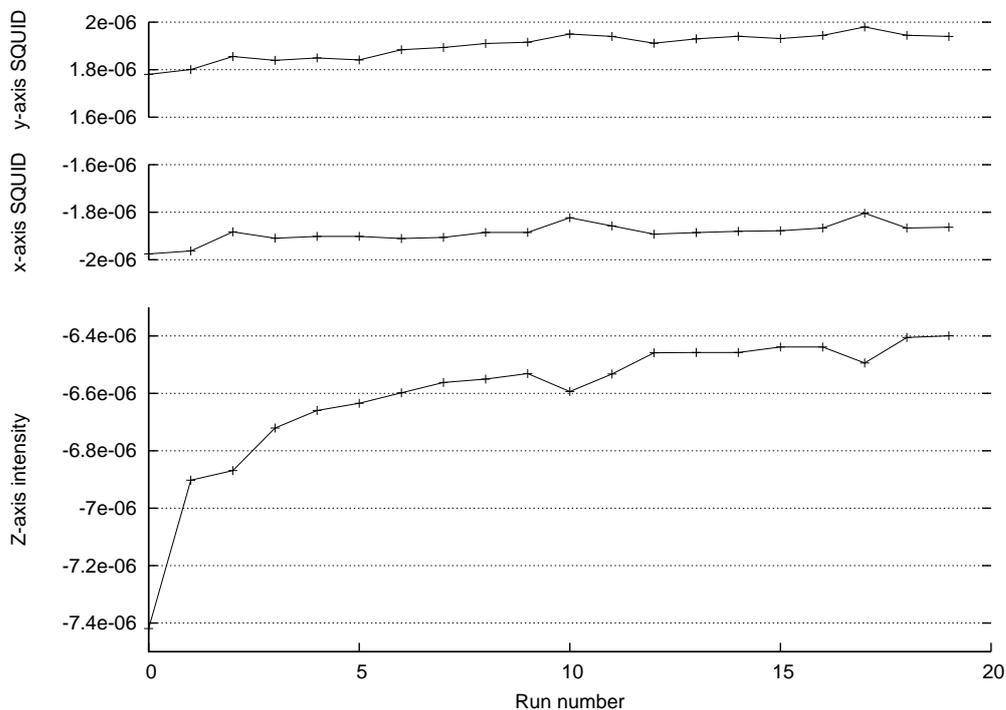
**Figure 3** 20 successive measurements of sample 1; output from the three SQUIDs plotted separately.
